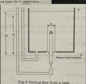
Consider the relationship of head loss  $(h_o-h_c)$  in vertical flow out of a tank. The ideal velocity in the plane of the vena contracta is
